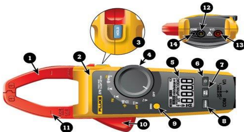
figure 2.27 clamp ammeter parts
