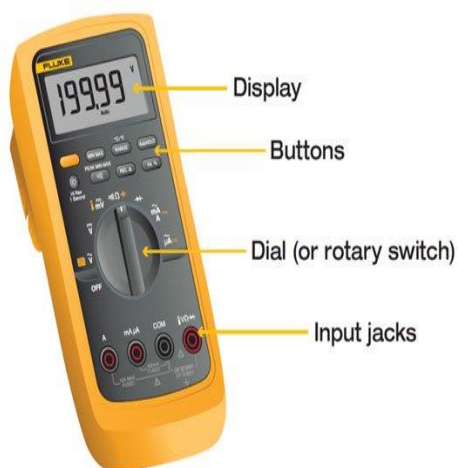
figure 2.24 components of multi meter
