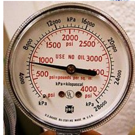
figure 2.28(a) Bourdon pressure gauge figure 2.28(b) reading psi(red scale) and kPa (black scale)
